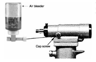
To replace a small amount of oil in the tool, connect tool to air line, remove cap screw (4), being sure NOT to cycle tool. Attach Cherry air bleeder 700A77 and cycle a number of times. This will insure the removal of any air from the hydraulic system and its replacement with fluid.
